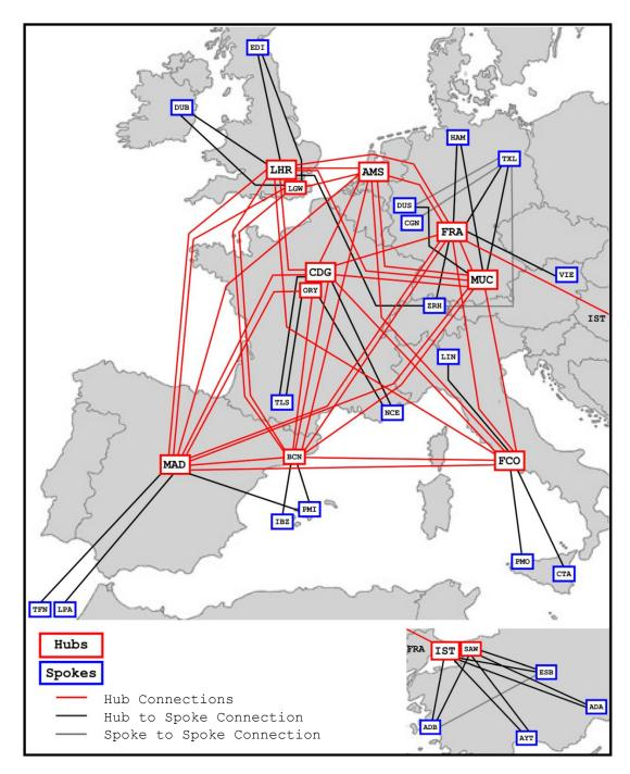
Figure 3: Considered complete flight network
